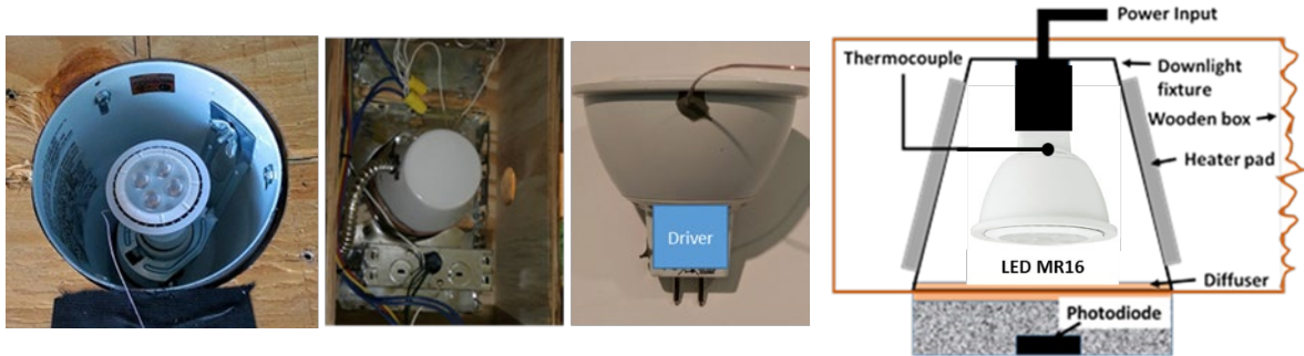
Figure A.7. Experiment setup for life test of LED MR-16 lamps.
